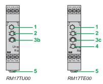
Un Green LED: indicates that supply to the product is on R Yellow LED: indicates relay output status
