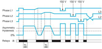
Tt: time delay after crossing of the threshold (adjustable on front panel)
