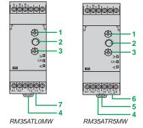
> Yellow LED: indicates relay output status (high temperature threshold)
