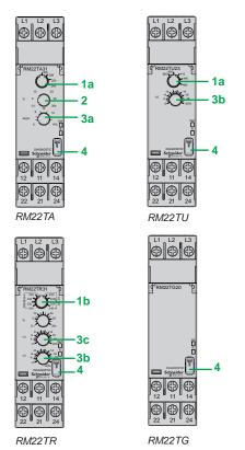
Green LED: indicates that supply to the product is on Yellow LED: indicates relay output status
