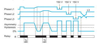
□ Control of overvoltage and undervoltage in window mode <U<
