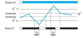
After a delay on pick-up after energization, and for as long as the temperature monitored by the PT100 probe remains between the two threshold settings on the front panel, the temperature relay R1 is closed.
