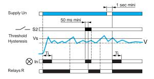
When relay RM35S has been configured in "memory" mode, if overspeed is detected, the output relay stays in the "open" state, irrespective of any further changes in the process speed.
