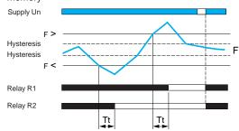
If "Memory" mode is selected, the relay opens after the time delay and stays in that position when crossing of the threshold is detected.
