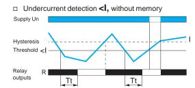
If the controlled current falls below the threshold setting for a time greater than that set on the front panel (0.1...30 s), the output relay opens and the R LED goes off. During the time delay, this LED flashes.
