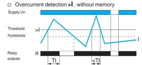
If the controlled current exceeds the threshold setting for a time greater than that set on the front panel (0.1...30 s), the output relay opens and the R LED goes off. During the time delay, this LED flashes.
