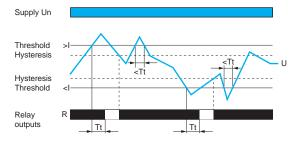
These relays operate in window mode where they check that the controlled current stays between a minimum and a maximum threshold.
